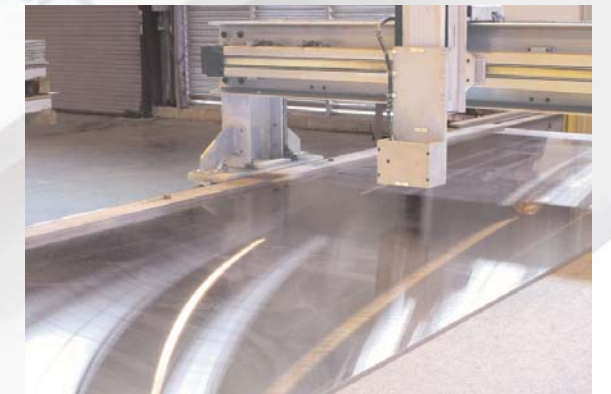
Laser equipment installed on this granite table checks MIC6 plates for flatness.
